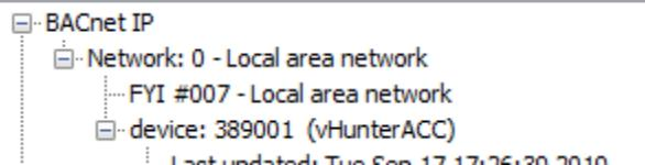
Once the device has been discovered, select it by clicking on the device 389001 , and right click to select DISCOVER again. This time check all the boxes to discover objects on the device.
